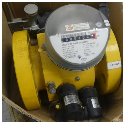
Figure 23. Detail of ELSTER TR22 G100 DN80 Class 600 turbine gas meter after the 100 mol% H 2 campaign
