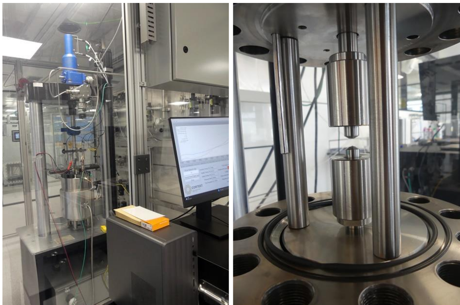
Figure 9. SSRT, fracture toughness and fatigue machine for testing in H 2 gas (left). Detail of fractured notched specimen (right)
