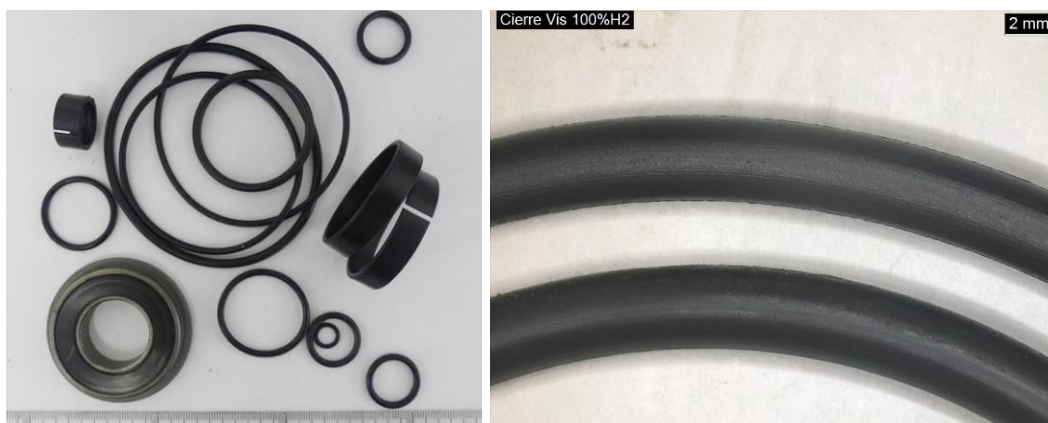
Figure 20. Parts of the pressure regulator (left) and detail of O-rings (right) after the 100 mol% H 2 campaign
