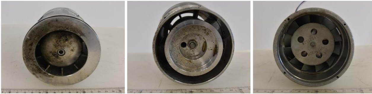
Figure 24. Detail of flow turbine gas meter bodies
