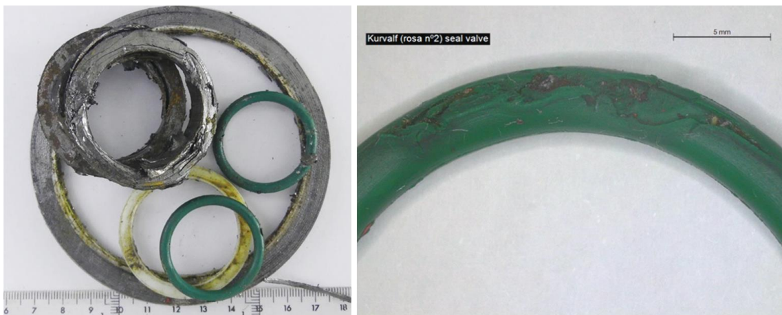
Figure 28. Components of the KURVALF rose n°2 plug valve and detail of O-ring after the 100 %mol H 2 campaign
