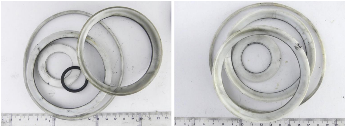
Figure 27. Components of the ALFA VALVOLE n° 5 (left) and ALFA VALVOLE n° 6 (right) Teflon seals after the 100 %mol H 2 campaign
