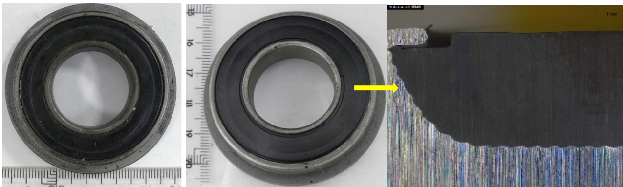
Figure 17. Valve seats tested at 20% H 2 + impurities of CO 2 and H 2 S (left) and 100 mol% H 2 (centre, right). The valve tested at 100 mol% H 2 was cut to verify the absence of blistering or other type of damage
