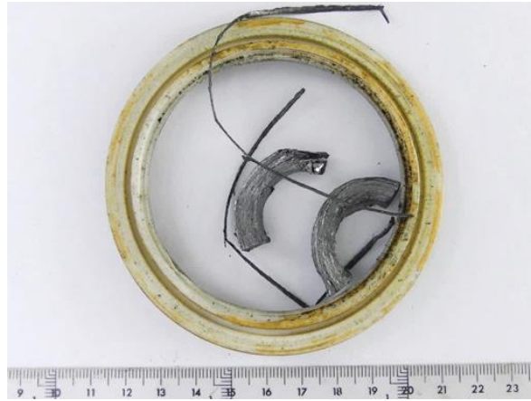
Figure 26. Components of the DIDTEK 600-3 valve showing detail of the graphoil and Teflon seals after the 100 mol% H 2 campaign
