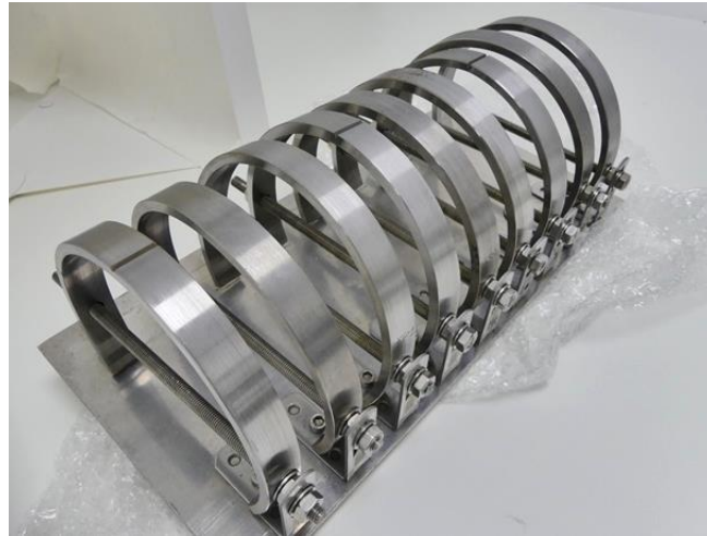
Figure 36. Detail of tested C-ring specimens after the 100 mol% H 2 campaign
