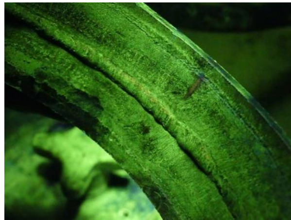
Figure 47. Magnetic particle testing of X52-X60 welded joint
