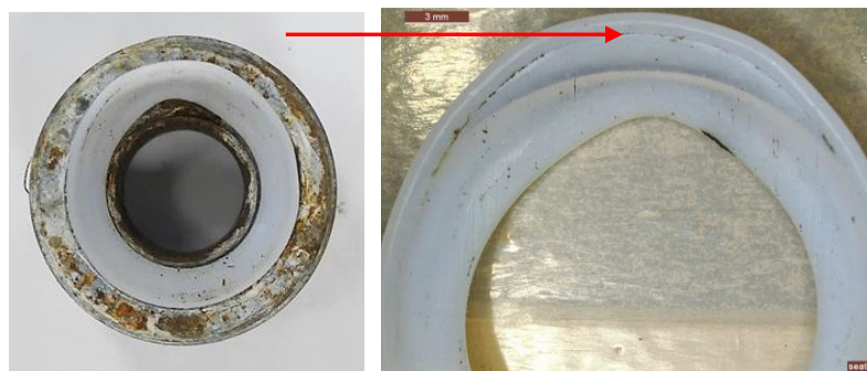
Figure 32. Photographs showing detail of the deformed TFM seat
