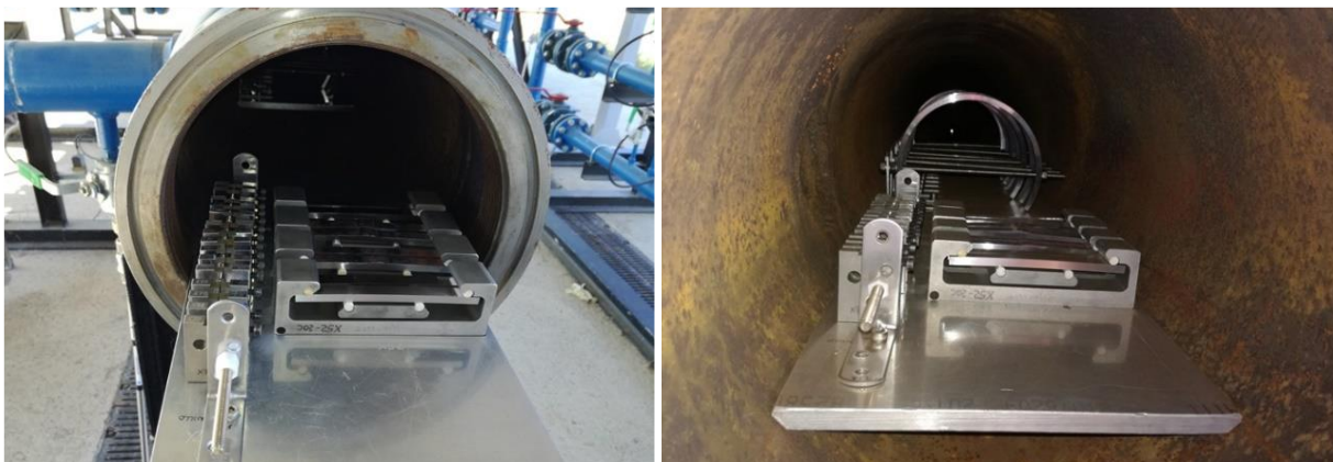
Figure 34. Test specimens inside the pig trap in the loop experimental platform at FHA at the beginning of the 2 nd experimental campaign (left) and once concluded (right)
