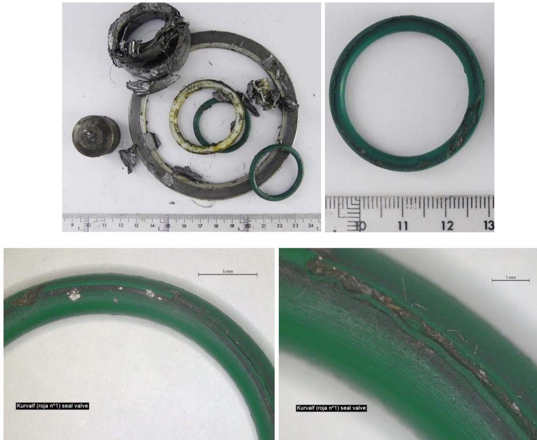
Figure 29. Components of the KURVALF red n°1 plug valve showing detail of O-rings after the 100 mol% H 2 campaign
