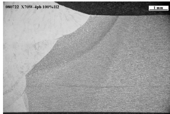
Figure 41. Optical micrograph of metallographic section of X70 welded joint after the 100 mol% H 2 experimental campaign
