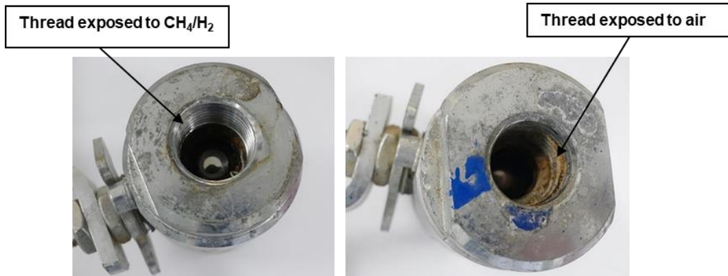
Figure 31. Photographs showing details of the ball valve
