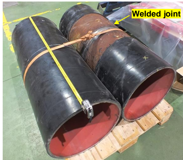
Figure 5. Detail of sections of the API 5L X70 steel pipes upon reception in Tecalia
