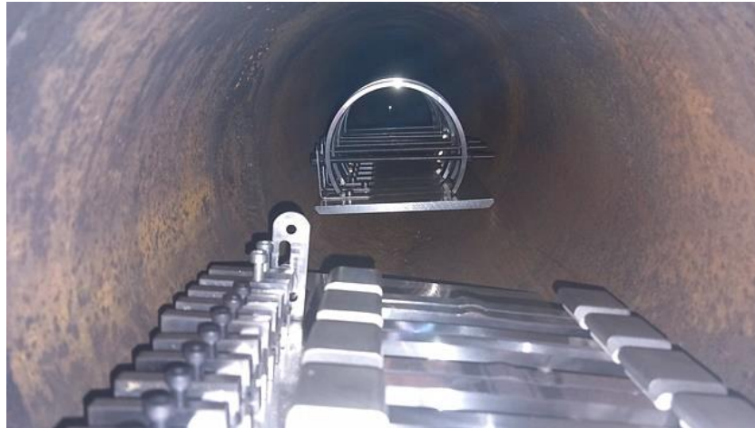
Figure 35. Test specimens inside the pig trap at the conclusion of the 100 mol% H 2 experimental campaign
