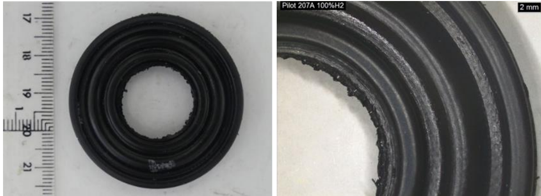
Figure 21. Detail of membrane from the pressure regulator after the 100 mol% H 2 campaign
