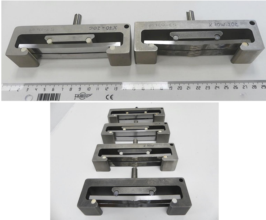
Figure 39. Tested X70 base and welded 4pb specimens supported in the loading jig after the 3 rd campaign (up) and tested x70 and X52 base and welded specimens after the 100 mol% H 2 campaign
