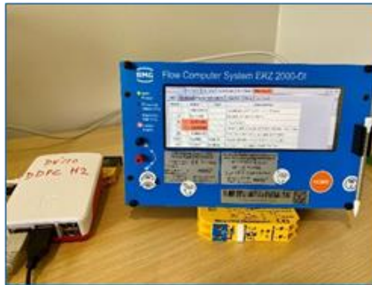
Figure 15: Example of correlative device communicating with the GCV to the flow-computer (Source: LC-Engineering)
