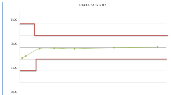
Figure 9: Flow calibration error curve with 99% H 2 (Source: GRTgaz)
