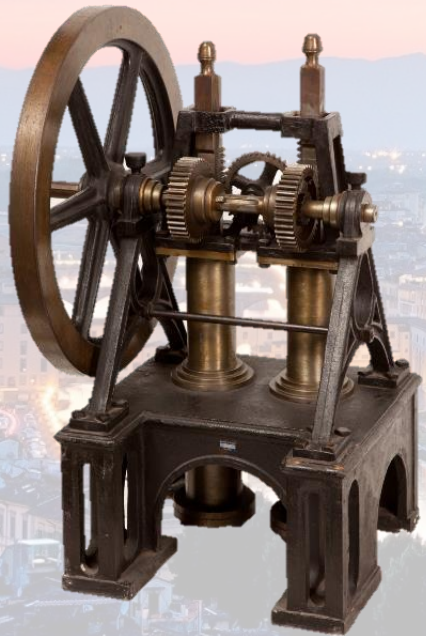
First combustion engine, running with H 2 , 1854
